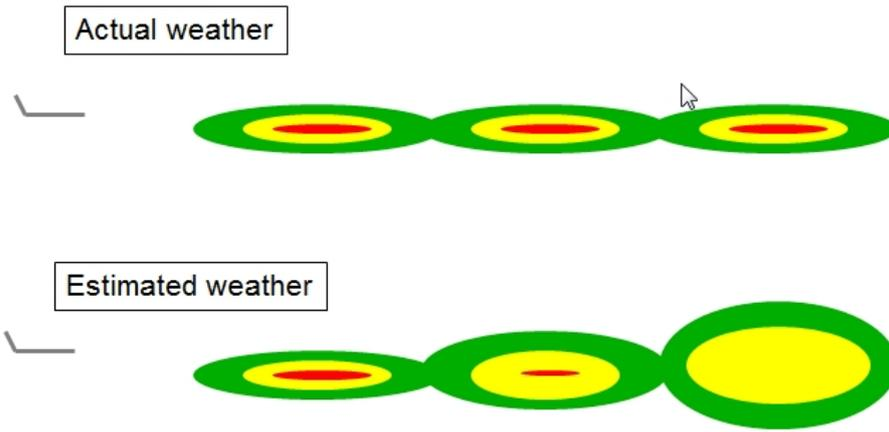
Another representation of this effect of angular resolution on range is given below, for aircraft fitted with on-path/off-path logic (Honeywell RDR-4000 on A320/A330/A340 family, and A350/A380 radars):
