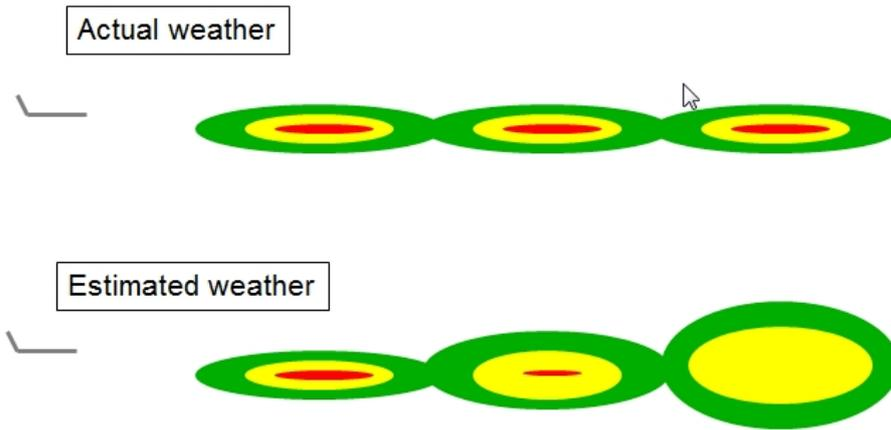
Another representation of this effect of angular resolution on range is given below, for aircraft fitted with on-path/off-path logic (Honeywell RDR-4000 on A320/A330/A340 family, and A350/A380 radars):
