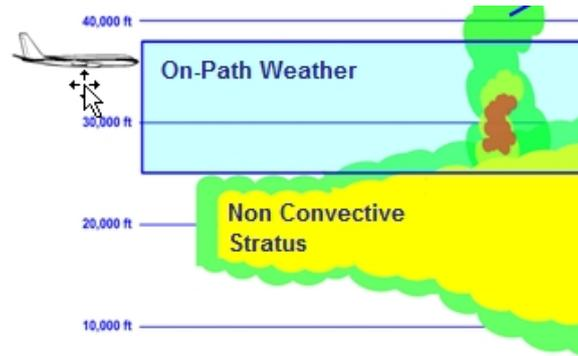
**This explains why cumuliform weather embedded in stratiform weather is difficult to see at high ranges.**
